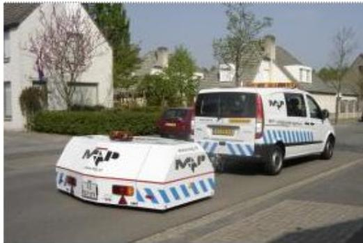
Figure 2 – An illustration of the close proximity method employed by M + P consulting engineers using a trailer lined with absorbent materials approximating anechoic conditions while also shielding aerodynamic noise [8]
